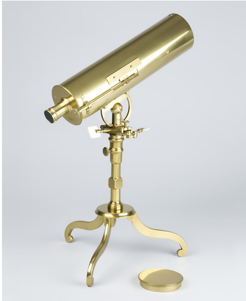
4. James Short, 1-foot Cassegrain reflecting telescope, c. 1758, Harvard University Collection of Historical Scientific Instruments (0053)
